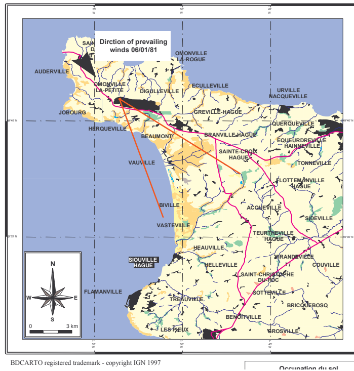
Figure 3.2.3.b: Map of the area under the prevailing winds at the time of releases associated with the silo fire (January 6 1981)
